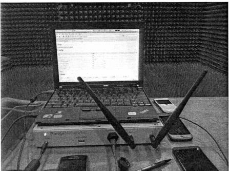
Figure 1: OpenBTS GSM/2G base station with inexpensive radio hardware (in anechoic chamber at CRC to avoid interference with deployed telecom services).
